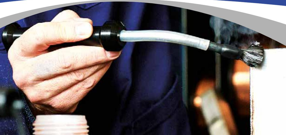
Cleaning and passivation of Stainless Steel welds in a single operation
